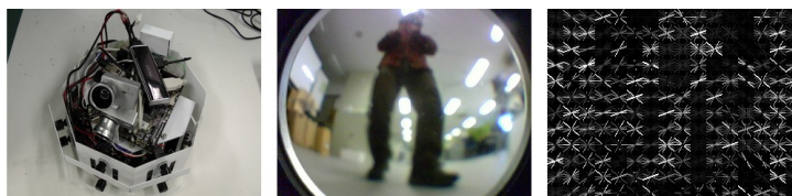
FIG. 1 – Our robot (left), an image taken by the robot (middle), its HOG representation (right)
